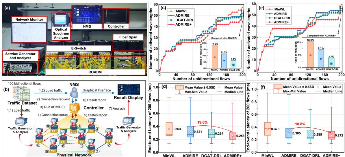
**Fig. 2:** (a) ADMIRE+ testbed, (b) Verification process, (c) No. of wavelength vs. No. of unidirectional flows in a 9-node topology, (d) End-to-end latency vs. 4 algorithms in a 9-node topology, (e) No. of wavelength vs. No. of unidirectional flows in GEANT, (f) End-to-end latency vs. 4 algorithms in GEANT.
