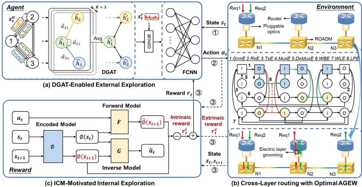
**Fig. 1:** Procedure of ADMIRE+. (a) DGAT-enabled external exploration, (b) Cross-layer routing with optimal AGEW, (c) ICM-motivated internal exploration.
