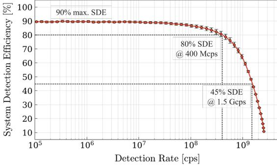
**Fig. 3: SDE as a function of detection rate** acquired with all 14 pixels active.
