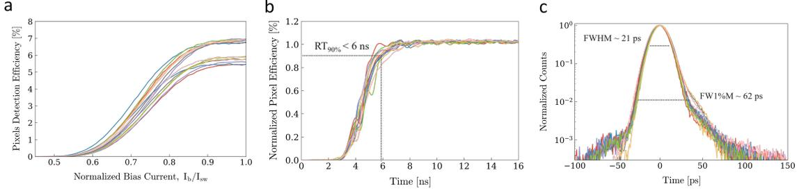
**Fig. 2: Single-pixels characterization.** **a**, Single-pixel detection efficiencies measured at 1550 nm as a function of the bias current. **b**, Recovery time measurement for the 14 individual pixels. The  $RT_{90\%}$  is lower than 6 ns for all pixels. **c**, Jitter measurement for the 14 pixels.
