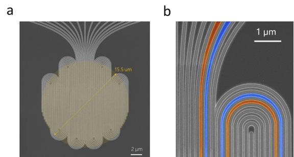
**Fig. 1: 14-pixel SNSPD array.** **a**, SEM image of the 14-pixel detector array. **b**, Recolored SEM image highlighting the path of two adjacent pixels.
