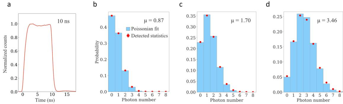
**Fig. 4: Photon-number resolution and state reconstruction with long pulses of light.** **a** Estimated profile retrieved from the counting histogram of a single pixel for 10 ns light-pulses. **b-d** Experimental and retrieved photon-counting statistics under Poissonian light illumination 10 ns light pulses.
