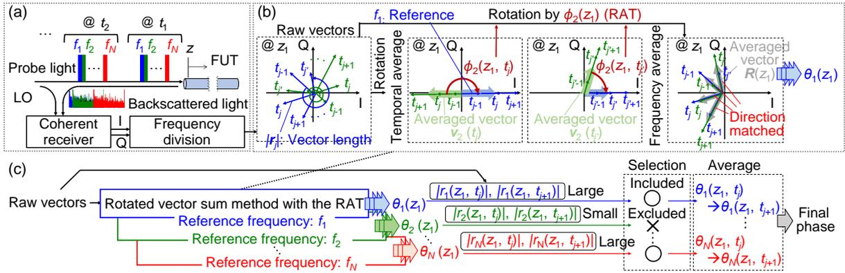
**Fig. 1:** Multi-frequency  $\Phi$ -OTDR DAS. The simplified schematic and the proposed phase calculation method.
