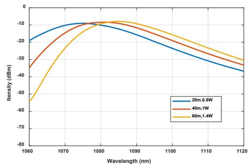
**Fig. 3:** Measured ASE spectra at different YDF lengths.
