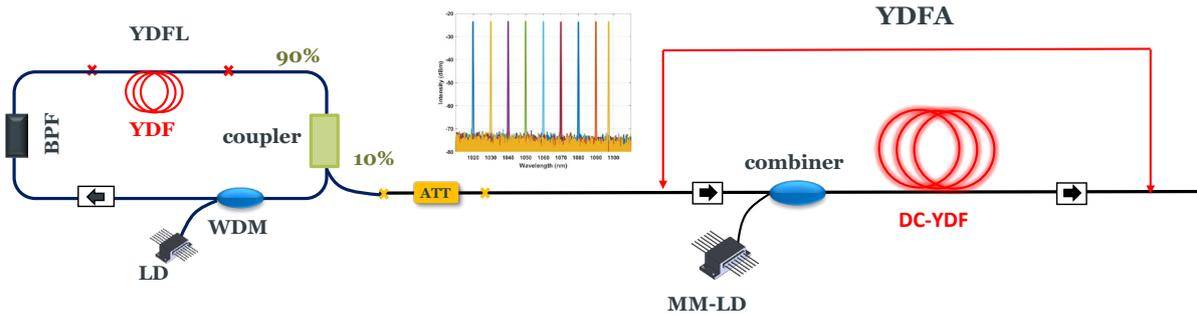
Fig. 4: Schematic of the long-wavelength YDFA in a cladding-pumped configuration.
