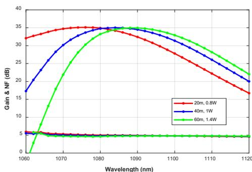
**Fig. 2:** Simulated gain and NF spectra of long-wavelength YDFA at 1060-1120 nm with different fibre lengths.
