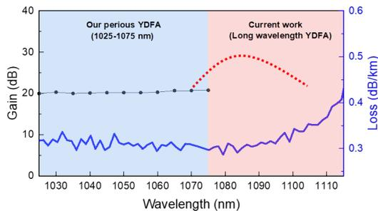
**Fig. 1:** Propagation loss of HCF at 1  $\mu\text{m}$  and YDFA performance in this window.
