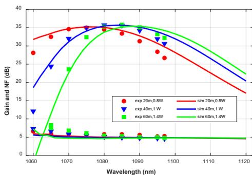
Fig. 5: Measured gain and NF spectra of the YDFA with various fibre lengths.
