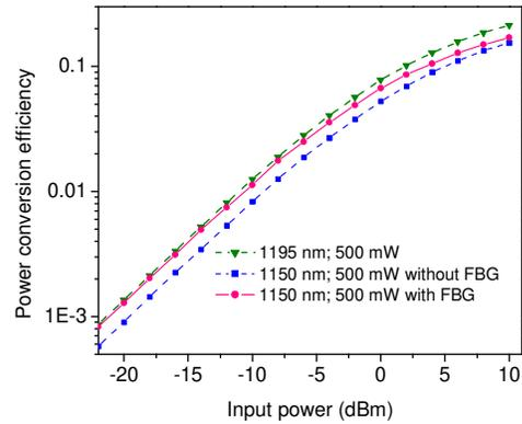
Fig. 6: Power conversion efficiency for both pumping schemes at 500 mW pump power.
