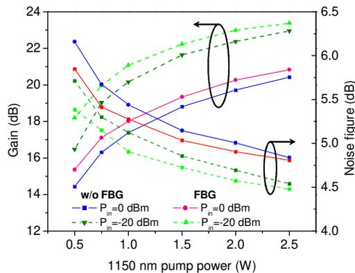
Fig. 5: Gain and noise figure for 915/1150 nm pumped BDFA with and without pump reflecting FBG
