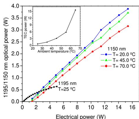
**Fig. 2:** Conversion stage and semiconductor LD output optical power vs. electrical power. Inset: Semiconductor LD TEC power as a function of ambient temperature.
