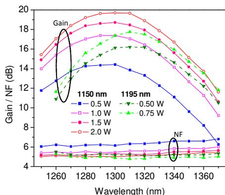
**Fig. 3:** Gain and noise figure for 0 dBm input signal power.
