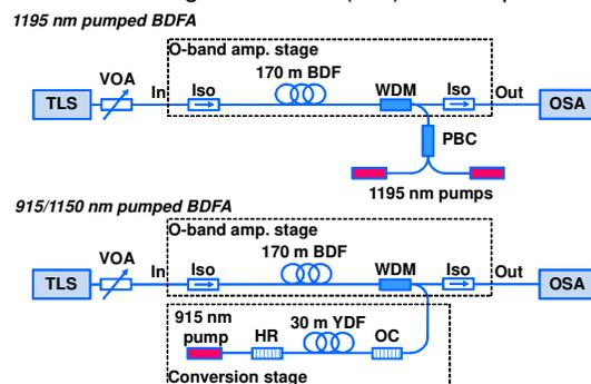
Fig. 1: 1195 nm (top) and 915/1150 nm (bottom) backward pumped BDFA designs; WDM: multiplexer; PBC: polarisation beam combiner; Iso: isolator.
