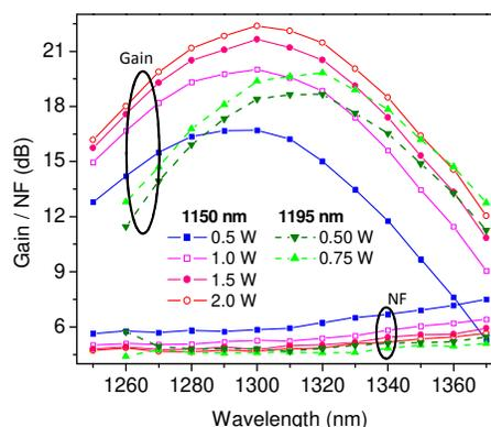
**Fig. 4:** Gain and noise figure for -20 dBm input power.
