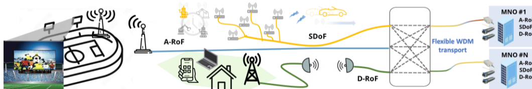
Fig. 1 Architectural layout of the proposed flexible, hybrid optical transport deployment including A-RoF, D-RoF, SDoF links.
