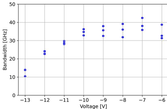
**Fig. 6:** Bandwidth measurement results at 1310 nm wavelength across 3 dies.
