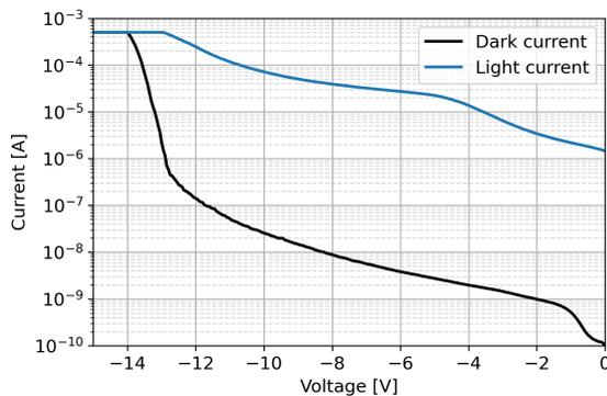
**Fig. 2:** Example of experimental dark and light I-V sweeps of the lateral APDs.
