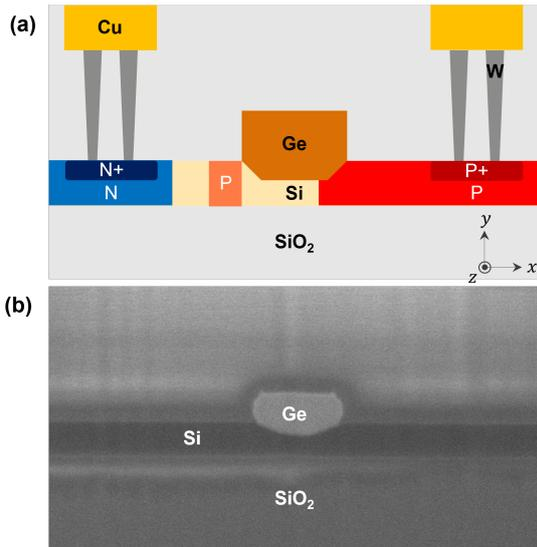
**Fig. 1:** Cross-section view schematics (a) and SEM image on Ge (b) of the lateral SACM APDs.
