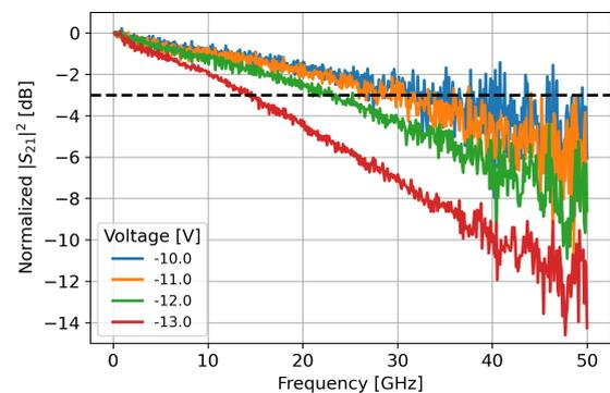
**Fig. 5:** Example of  $S_{21}$  measurement results for different applied DC voltages.
