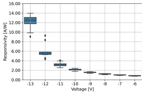
**Fig. 4:** Wafer-scale responsivity measurement results at 1310 nm wavelength across 14 dies.
