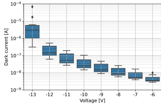
**Fig. 3:** Wafer-scale dark current measurement results across 14 dies.
