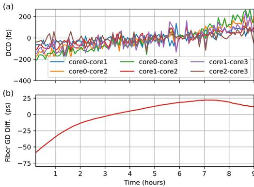
**Fig. 3:** (a) Differential core delay (DCD) averaged over the 12 THz measurement bandwidth during the 9 h long measurement. The observed core-to-core delay is changes with  $<420$  fs. (b) The corresponding group delay change for the fiber. The change is about 2 orders of magnitude larger than the relative core-to-core delay of the multi-core fiber.
