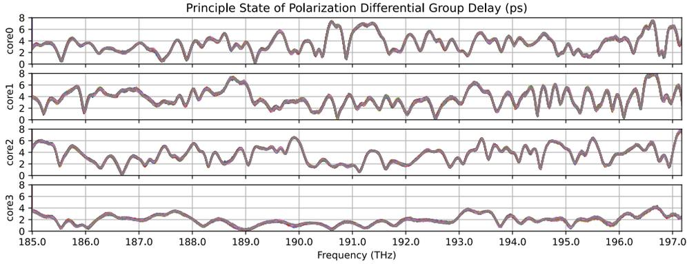
**Fig. 2:** Measurement of the differential group delay (DGD) for all four cores within the 6.3 km long 4-core multi-core fiber. The measurements show overlaid traces taken about 5 mins apart during a 9-hour time window, verifying that the observed DGD is stable over long time scales. However, the observed ps-level DGD implies that the observed propagation time will be highly sensitive to any change in input state-of-polarization.
