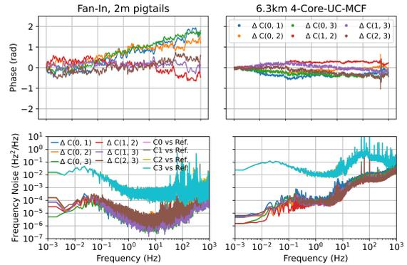
**Fig. 4:** (Top) Phase evolution and (Bottom) frequency noise spectrum, between all core-core combinations of a fan-in with 2m pigtails in the lab (left) and the 6.3 km multi-core fiber (right). A difference of 2 and 4 orders of magnitude is observed at a frequency of 1 Hz and 10 mHz, respectively.
