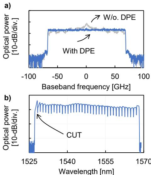
Fig. 2. a) Optical spectrum of the 135-GBaud DP-PCS-64QAM signal at the transmitter output. b) DWDM spectrum with the channel under test at 1527.66-nm.
