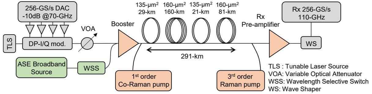
Fig. 1. 291-km unrepeated transmission link.
