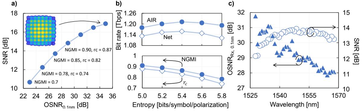
**Fig. 3.** Experimental results. a) Back-to-back: sensitivity to noise of the 135-GBaud DP-PCS-64QAM signal. b) Transmission: PCS-64QAM entropy optimization with the channel under test at 1554.09-nm. c) Optical signal to noise ratio and signal-to-noise ratio after transmission.
