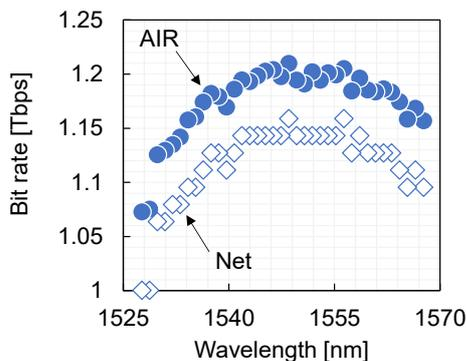
**Fig. 4.** Bit rate measured as a function of wavelength after 291-km.
