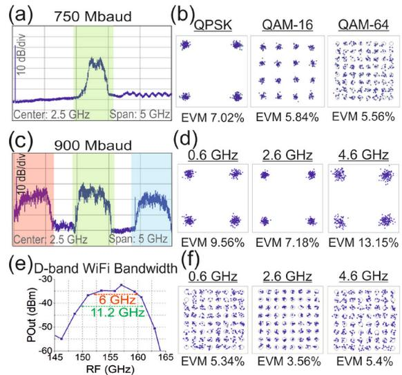
**Fig. 3:** Experimental results of the D-band WiFi link: (a) RF spectrum of a 750 MBd single band, (b) constellation diagrams and EVM value of QPSK, QAM-16, QAM-64, (c) RF spectrum of a 900 MBd transmission of 3 bands at 0.6 GHz, 2.6 GHz, 4.6 GHz, (d) constellation diagrams and EVM values of each QPSK-band (e) bandwidth characterization of the FiWi link, (d) three band 64-QAM transmission.
