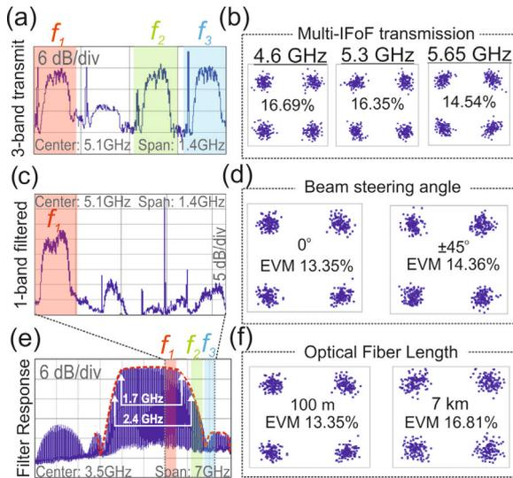
**Fig. 4:** Experimental results of the WiFiWi link, including: (a) RF spectrum of a 250 Mbaud 3-band transmission, and (b) respective constellation diagrams, (c) RF spectrum of the same transmission using a filter to select the first band, (e) filter's frequency response, constellation diagrams and achieved EVM values for filtered transmission, (d) with and without beamsteering and (f) at different fiber lengths.
