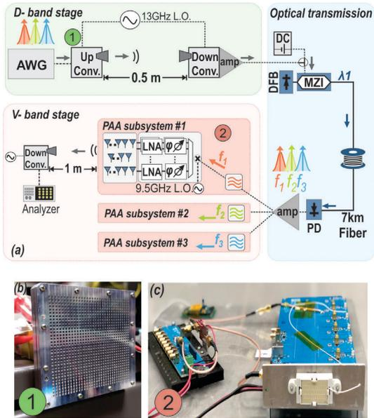
**Fig. 2:** (a) Experimental Setup of the proposed system including close up pictures of (b) Sub-THz (D-Band) Tx antenna and (c) V-band MIMO Tx antenna.
