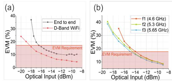
**Fig. 5:** Experimental characterization of the dynamic range: a) the Sub-THz FiWi link and the end-to-end WiFiWi link for a single band, and b) equal EVM-performance of the three end-to-end WiFiWi links versus the power reaching the PD.
