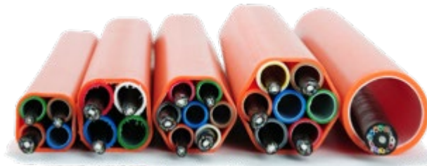
Fig. 1: Left: Microduct bundle configurations with micro cables. Right: Standard 1.25" duct with a standard loose tube cable. Increases of more than twice the fibre in the same space can be achieved with microduct bundles and micro cables.
