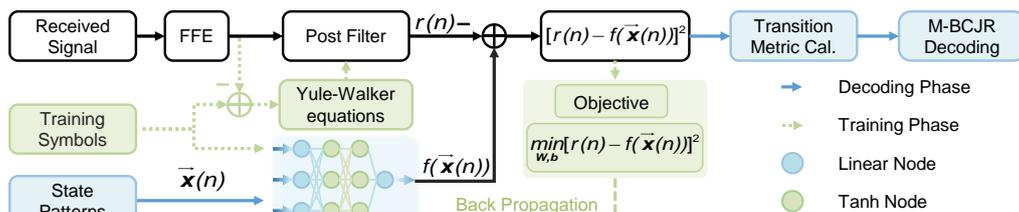
**Fig. 1.** The block diagram of the DNN-MBCJR equalization scheme, with DNN as the nonlinear channel response estimator and simplified MBCJR decoder for the reduction of overall complexity.
