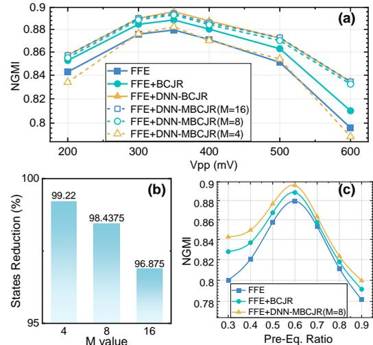
**Fig. 3:** The NGMI versus (a) the Vpp and (c) the pre-equalization ratio for a 140GBaud PAM-8 signal in B2B case. (b) is the percentage of states reduction for DNN-MBCJR algorithm with different M value
