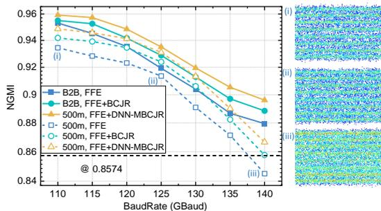
Fig. 5: The NGMI versus the baud-rate for a 140-Gbaud PAM-8 signal at 6-dBm ROP
