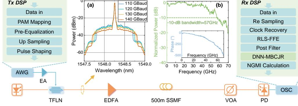
**Fig. 2:** Experiment setup for the ultra-high baud-rate PAM-8 IM/DD transmission over 0.5-km SSMF with the detailed DSP blocks. The inset (a) shows the measured optical spectra of PAM-8 signals for different baud-rates after electro-optical conversion, and the inset (b) represents the frequency response of overall system for B2B case.
