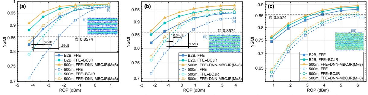
Fig. 4 The NGMI versus ROP for (a) 140-Gbaud PAM-4, (b) 140-Gbaud PAM-6 and (c) 140-Gbaud PAM-8
