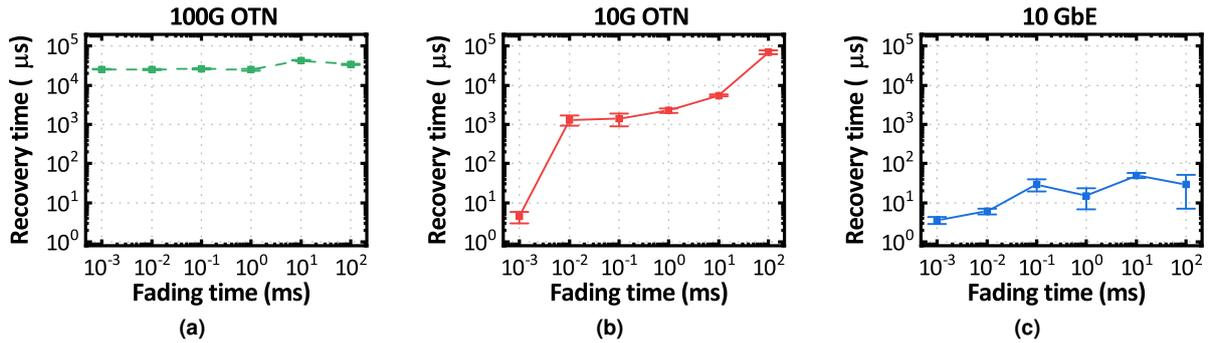
Fig. 2: Measured recovery times vs. fading time for the three different transmission protocols: (a) 100G using OTN; (b) 10G using OTN; (c) 10G Ethernet transceiver.
