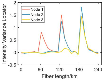
**Fig. 4:** Intensity variance locator curves for several insufficient EDFA amplifications.
