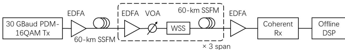
**Fig. 2:** Simulation setup. Tx: transmitter, EDFA: erbium-doped fiber amplifier, SSMF: standard single-mode fiber, VOA: variable optical attenuator, WSS: wavelength selection switch, Rx: receiver, DSP: digital signal processing.
