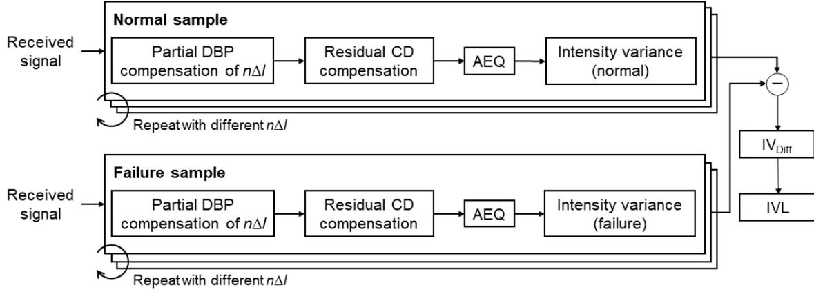
**Fig. 1:** Framework of the proposed intra-node failure localization scheme. DBP: digital back-propagation, CD: chromatic dispersion, AEQ: adaptive equalizer;  $IV_{Diff}$ : difference between the intensity variances of the normal and failure samples; IVL: intensity variance locator.
