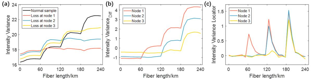
**Fig. 3:** Localization of the excess attenuations of WSSs at different nodes. (a) intensity variance curves; (b) differences between intensity variances for the normal and failure samples; (c) intensity variance locator curves.
