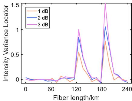
**Fig. 5:** Intensity variance locator curves for several excess WSS attenuations.
