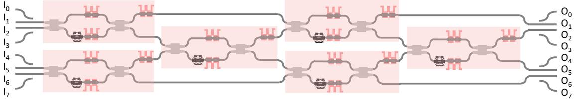
**Fig. 2:** A  $8 \times 8$  Transverse Mode Encoded Programmable Quantum Processor build on a Clement mesh. This processor can perform an  $8 \times 8$  unitary matrix transformation with only six MZIs.
