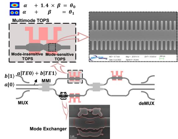
**Fig. 1:** A Schematic illustration of  $4 \times 4$  building block for the Transverse Mode Encoded Programmable Quantum Processor. The block includes a multimode TOPS consisting of a mode insensitive and a mode-sensitive TOPS. It also includes a mode exchanger to convert TE0 to TE1 and vice versa.
