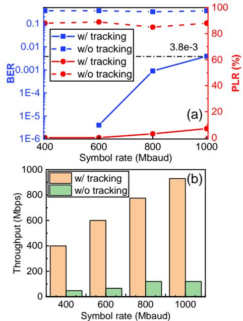
**Fig. 3:** (a) BER and PLR performance and (b) throughput versus symbol rate of OOK signals with a wave ASCR of 0.103 rad/s, moving speed of 8 cm/s, moving range of 10 cm, and 1.6-m air path.
