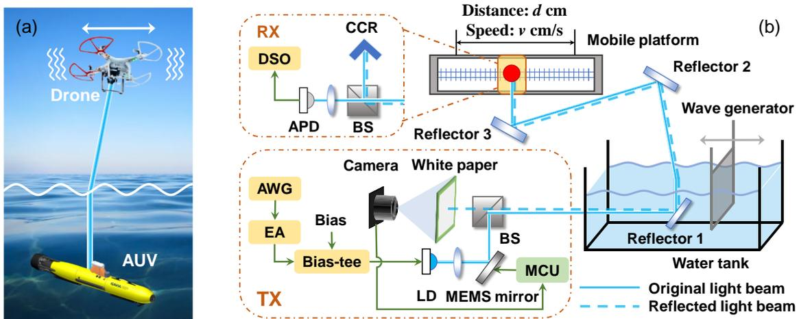
**Fig. 1:** (a) Illustration of water-air OWC link between an autonomous underwater vehicle (AUV) and drone and (b) Proposed imaged-based beam tracking for a water-air OWC system with the mobile receiver through a wavy water-air interface.
