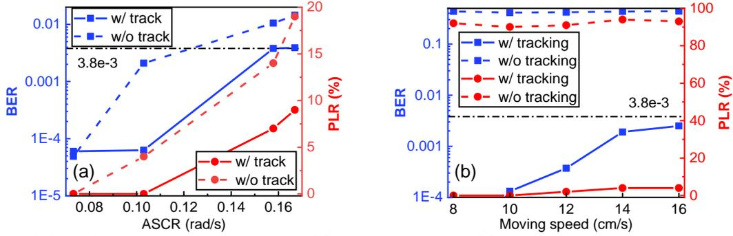
**Fig. 2:** BER and PLR performance of 800-Mbaud OOK signals versus (a) ASCR with a stationary receiver and 1.4-m air path and (b) moving speed with no wave added, 20-cm moving range, and 1.6-m air path.
