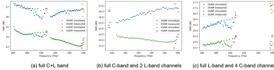
**Fig. 4.** Model simulation and measured results comparison: OSNR and GSNR of each channel at the receiver
