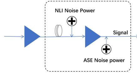
Fig. 2: .The transmission link model scheme
