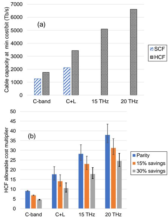
Fig. 3: Case 3. a) Cable capacity values for minimum cost/bit systems, b) maximum HCF cost multiple.
