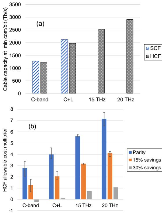
Fig. 1: Case 2a. a) Cable capacity values for minimum cost/bit systems, b) maximum HCF cost multiple.
