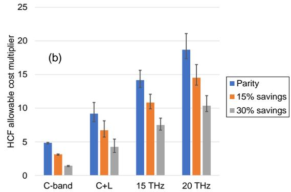
Fig. 2: Case 2b. a) Cable capacity values for minimum cost/bit systems, b) maximum HCF cost multiple.
