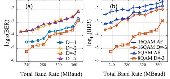
**Fig. 5:** BER versus the total baud rate of the two users for (a) the proposed method using 8QAM under different  $D$ , (b) the proposed method under  $D=-3$  and conventional AF-PNC.
