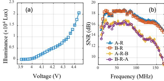
**Fig. 4:** (a) The illuminance versus voltage for the LD. (b) the measured SNRs for the links A-R, B-R, A-R-B, and B-R-A.
