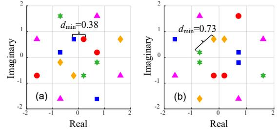
**Fig. 2:** (a) Classification results and  $d_{min}$  when  $(\alpha, \beta)$  is (a)  $(1, 1+i)$  and (b) the optimal  $(1, i)$ .  $D=-1$ ,  $h_A = 0.9 \cdot \exp(j\pi/4)$ , and  $h_B = 1$ . The formats at users A&B are 4QAM. The superposed signal  $y_R$  has 16 points, which are classified into five groups.
