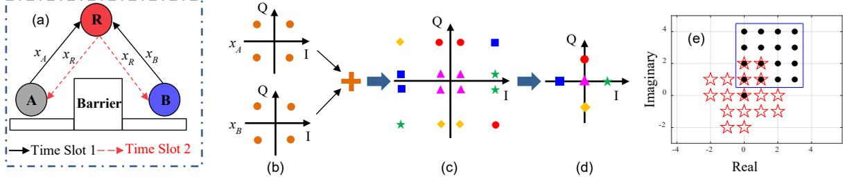
**Fig. 1:** (a) PNC scheduling in TWRN; (b) 4QAM constellations of an OFDM subcarrier at nodes A and B; (c) The superposed signal at the relay R. 16 superposed points are categorized into 5 groups  $u(x_A, x_B)$ ; (d) Constellation of re-encoded  $x_R$ ; (e) Two sets (stars and dots) of representative elements for  $Z(\xi)/(4+i)$  when  $D=-1$ . The dots in the blue square are selected as 16QAM.
