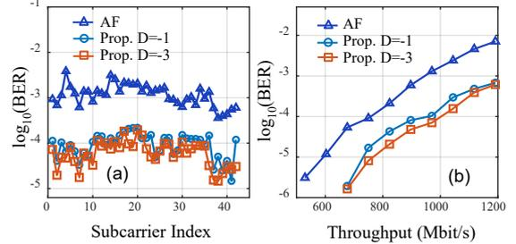
**Fig. 7:** BER versus (a) the subcarrier index at 1.014 Gbit/s, and (b) the throughput for adaptively-loaded OFDM.
