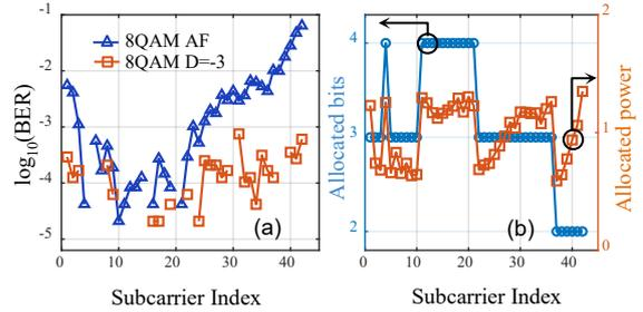
**Fig. 6:** (a) BER versus the subcarrier index when the total baud rate is 309 Mbaud using 8QAM under  $D=-3$ . (b) bit-and-power loading results using Chow's algorithm at 0.97 Gbit/s.
