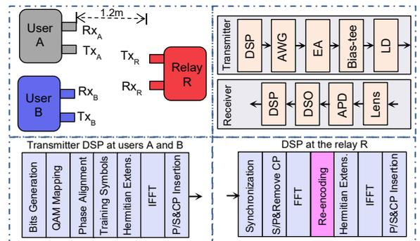
**Fig. 3:** Experimental setup. AWG: arbitrary waveform generator; EA: electrical amplifier; LD: laser-diode; APD: avalanche photo-diode; DSO: digital storage oscilloscope.
