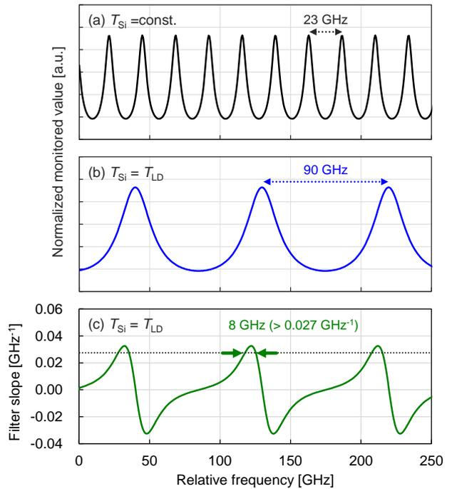
**Fig. 3:** Calculated results of wavelength locker output. (a)  $T_{Si} = \text{const.}$ , (b)  $T_{Si} = T_{LD}$ , (c) filter slope.
