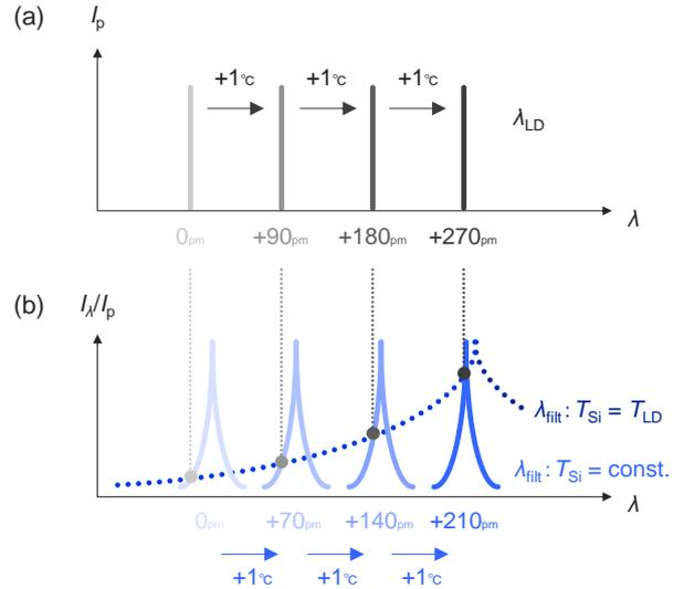
**Fig. 2:** Temperature characteristics of wavelength locker. (a) Lasing characteristics, (b) Filter characteristics.
