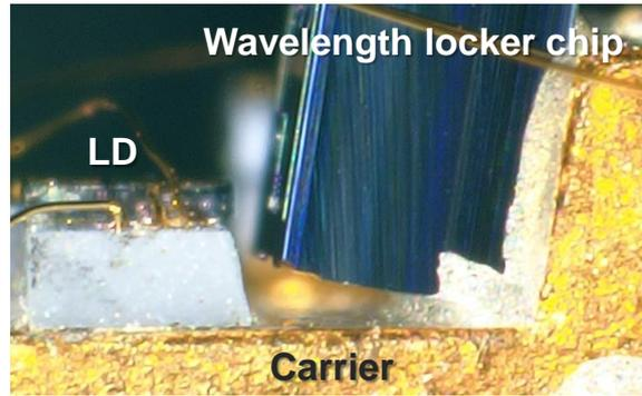
Fig 4. Fabricated optical sub-assembly.
