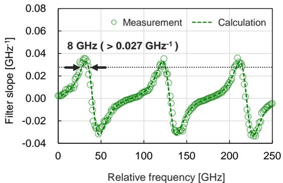
Fig 6. Slope characteristics of wavelength locker output.
