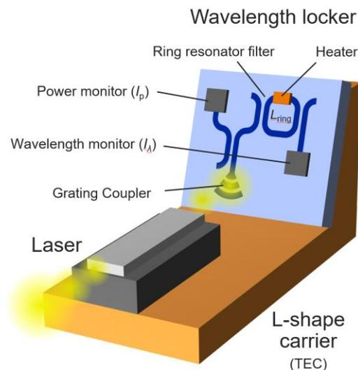
Fig. 1: Schematic diagram of laser optical sub-assembly.
