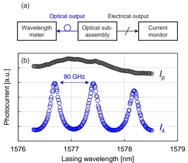
Fig 5. Measured characteristics of wavelength locker.
