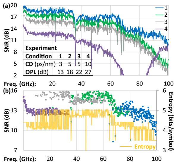
**Fig. 3:** Link diversity experiment: (a) the 4 link conditions and their SNR profiles; (b) SC allocations per cluster of users by EL-SCG and the overall entropy profile of all subcarriers.
