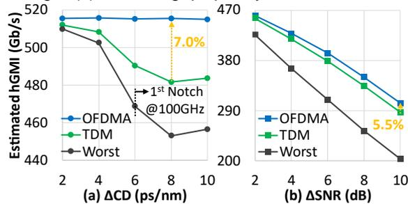
**Fig. 2:** hGMI with different (a) CD and (b) OPL. The 1<sup>st</sup> CD fading notch appears at 100 GHz when  $CD \approx 6$  ps/nm; “Worst”: all the users operate at the worst case without rate adaptation.
