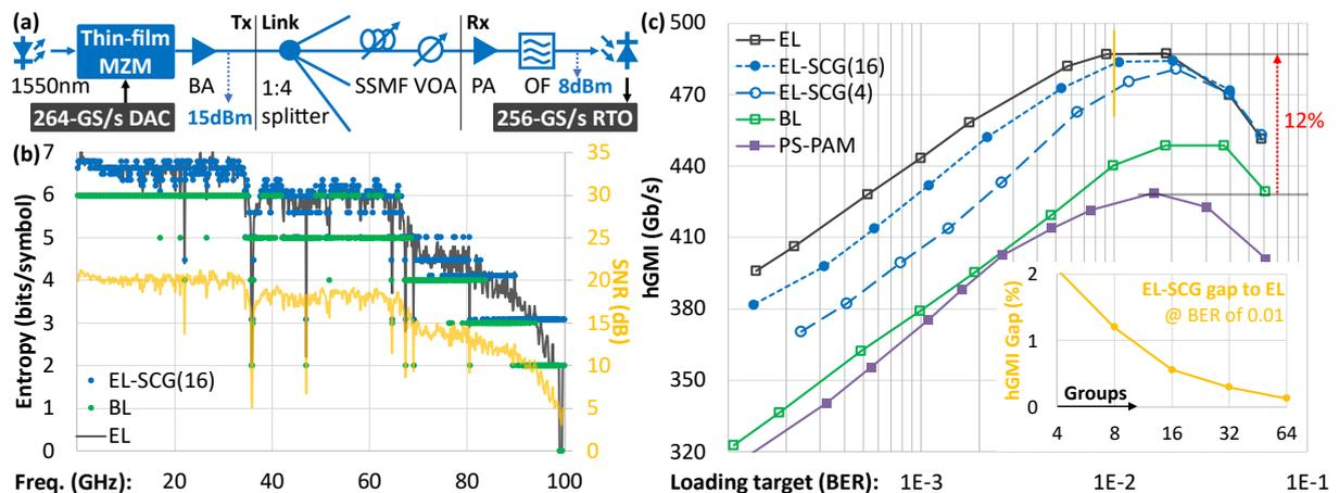
Fig. 1: (a) Experimental setup [18]; the 264-GS/s D/A converter (DAC) is made by digital-band interleaving (DBI) of 3x88-GS/s DACs; BA/PA: booster-/pre-amplifier; RTO: real-time oscilloscope. Rate comparison with a fixed link condition (5-ps CD, 8-dBm received optical power): (b) SNR and entropy profiles, (c) hGMI; (c-inset) shows the gap of EL-SCG to EL.
