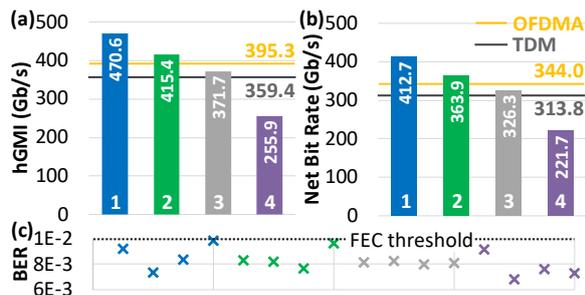
**Fig. 4:** Achievable rates for each link condition (bars) and the aggregated rates of all users evaluated by (a) hGMI and (b) net bit rate after a 20% HD-FEC; (c) the BER is below the threshold of 0.01 for all 16 OFDMA users.
