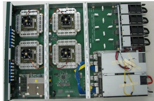
Fig. 8: Photograph of a switch server accommodating 4 CPO daughter boards.
