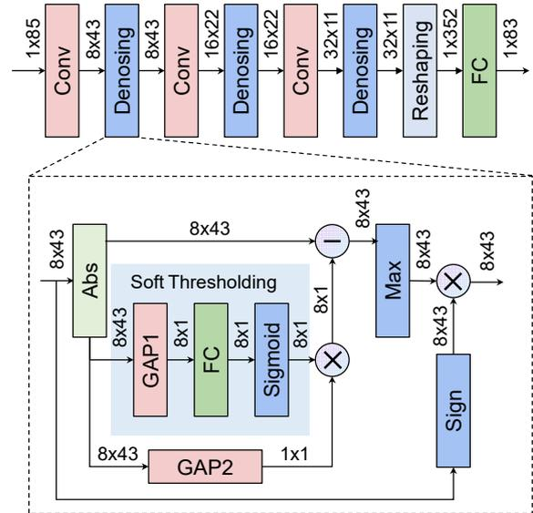
Fig. 2: The structure of the proposed EDFA gain model based on CNN with inserted denoising layers.
