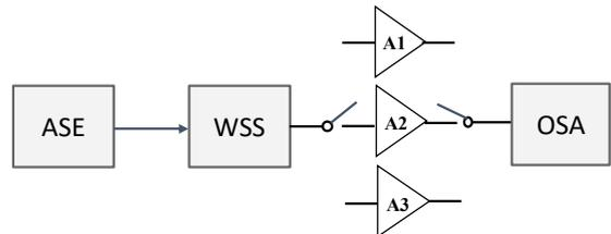
Fig. 1: Experimental setup for collecting datasets. ASE: Amplified Spontaneous Emission, WSS: Wavelength Selective Switch, Optical Spectrum Analyzer.
