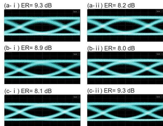
**Fig. 4:** 25 Gb/s NRZ eye patterns (BTB) of the module working at (a) 1540 nm, (b) 1550 nm, and (c) 1560 nm, respectively. Column ( i ) indicates eye patterns of the incident light at TE-polarization; Column ( ii ) indicates eye diagrams of the incident light at TM-polarization.
