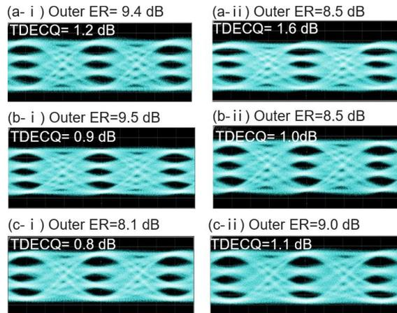
**Fig. 5:** 50 Gb/s PAM4 eye patterns (BTB) of the module working at (a) 1540 nm, (b) 1550 nm, and (c) 1560 nm, respectively. Column (i) records eye patterns of the incident light at TE-polarization; Column (ii) records eye diagrams of the incident light at TM-polarization.
