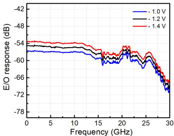
**Fig. 3:** Measured small-signal frequency responses of the PIM module at different bias voltage.
