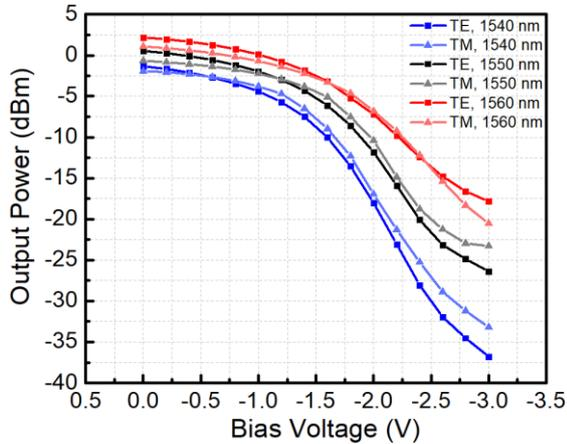
**Fig. 2:** Static extinction ration of the PIM module versus reverse bias voltage for several wavelengths at TE and TM polarizations
