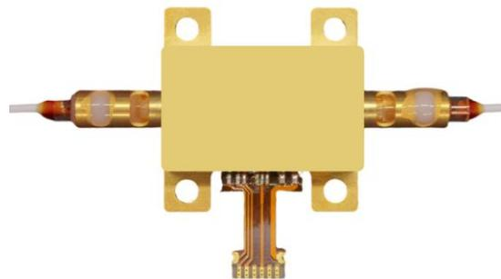
**Fig. 1:** Picture of a packaged PIM module with a FPC interface
