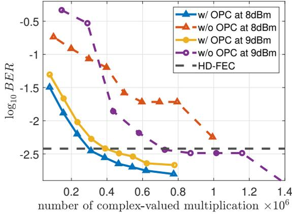
Fig. 2: BER achieved for different CC values for 2 datasets where optical solutions -OPC- are used and 2 where not. 2 launch powers are considered : 8 dBm and 9 dBm
