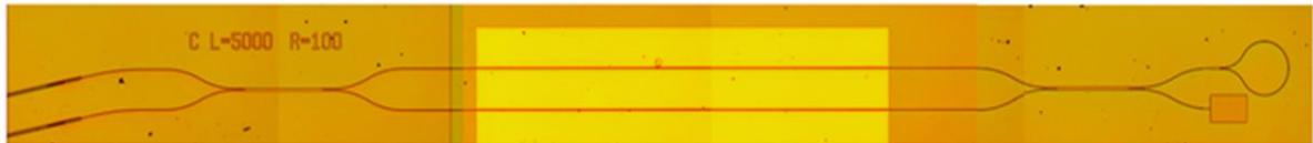
Fig. 4: The fabricated amplitude controller based on Mach Zehnder interferometer and total reflector with ring mirror.
