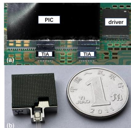
**Fig. 1:** Photographs (a) inside and (b) outside of the IC-TROSA.
