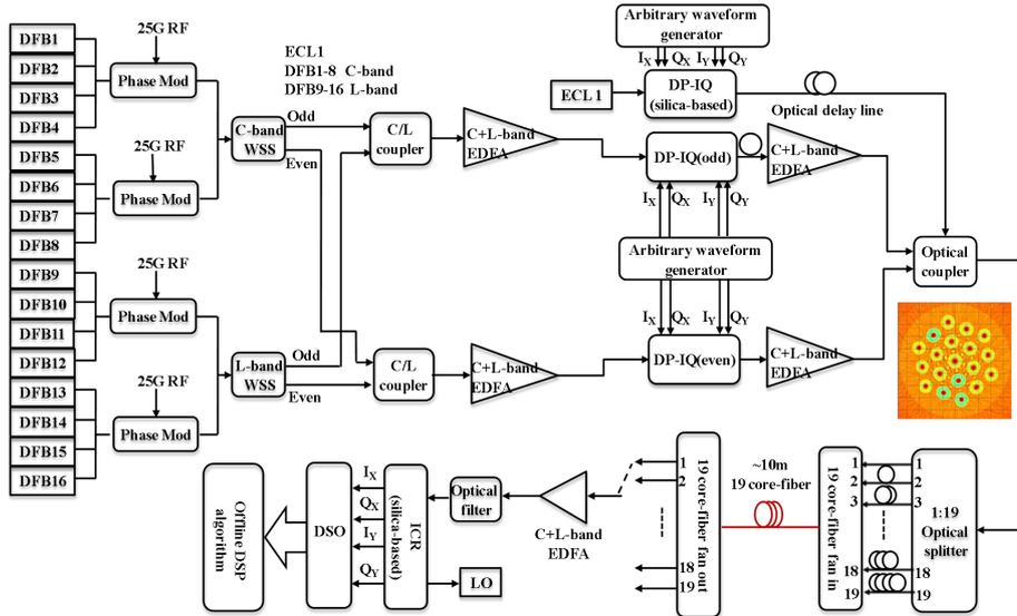
Fig. 3: Experimental set-up for 1.06 Pb/s transmission in a 19-core fiber.
