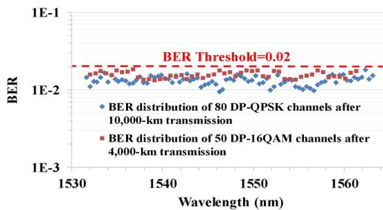
Fig. 5: Measured curve of all the BER of the transmission signals before and after 10000 km and 4000 km transmission.
