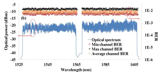
Fig. 4: Max, min and average BER of the 19 spatial channels for the 375 measured wavelengths with optical spectrum.
