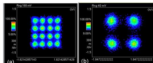
**Fig. 2:** Constellation diagram of (a) 85GBaud 16-QAM and (b) 100GBaud QPSK.
