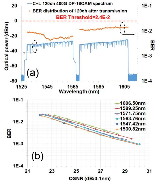
Fig. 6: (a) Transmission performance and spectrum of 120-ch; (b) Back-to-back BER performance at selected wavelength.
