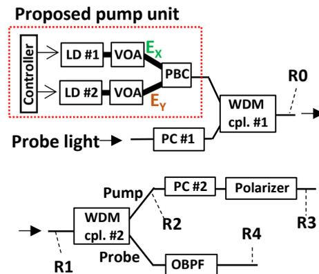
Fig. 1: Proposed pump unit and experimental setup.
