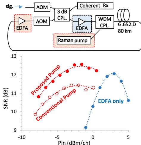
**Fig. 5:** Experimental setup for data transmission (only main components) and measured power tolerance. Red: fwd pumped Raman used, Blue: only EDFA used.
