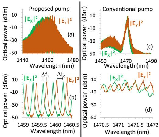
**Fig. 2:** The measured optical spectra of the pump light. (a) and (b) : proposed pump unit, (c) and (d) : commercially available pump unit, for comparison.
