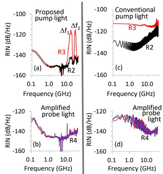
**Fig. 4:** Measured RIN. (a), (b): proposed pump light at R2-R3, amplified probe light at R4. (c), (d): conventional pump light at R2-R3, amplified light at R4
