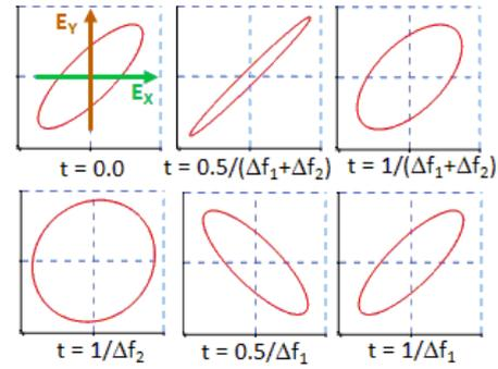
**Fig. 3:** Simulated Lissajous figures of  $E_x$  and  $E_y$  of pump light before transmission.
