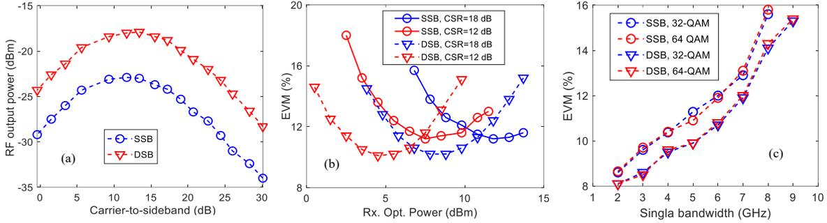
**Fig. 4:** System performance: (a) output 100-GHz signal; (b) OFDM signal vs rx. opt. power at AP; (c) vs signal bandwidth.
