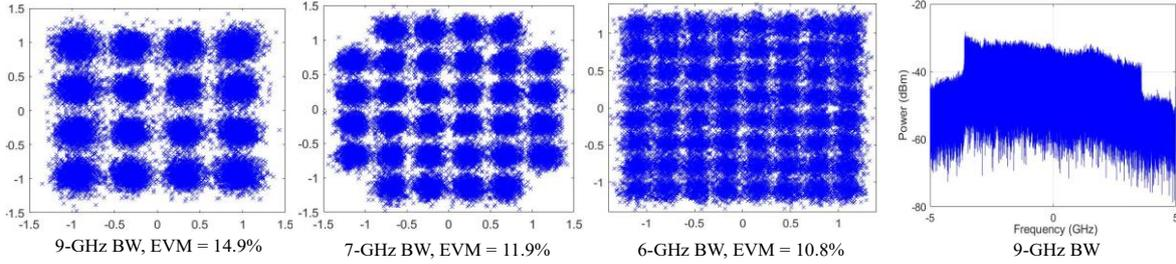
**Fig. 5:** Examples of constellations and spectrum of received signal.
