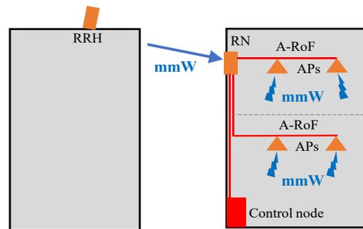
Fig. 1: RoF system for relaying mmW radio signal.
