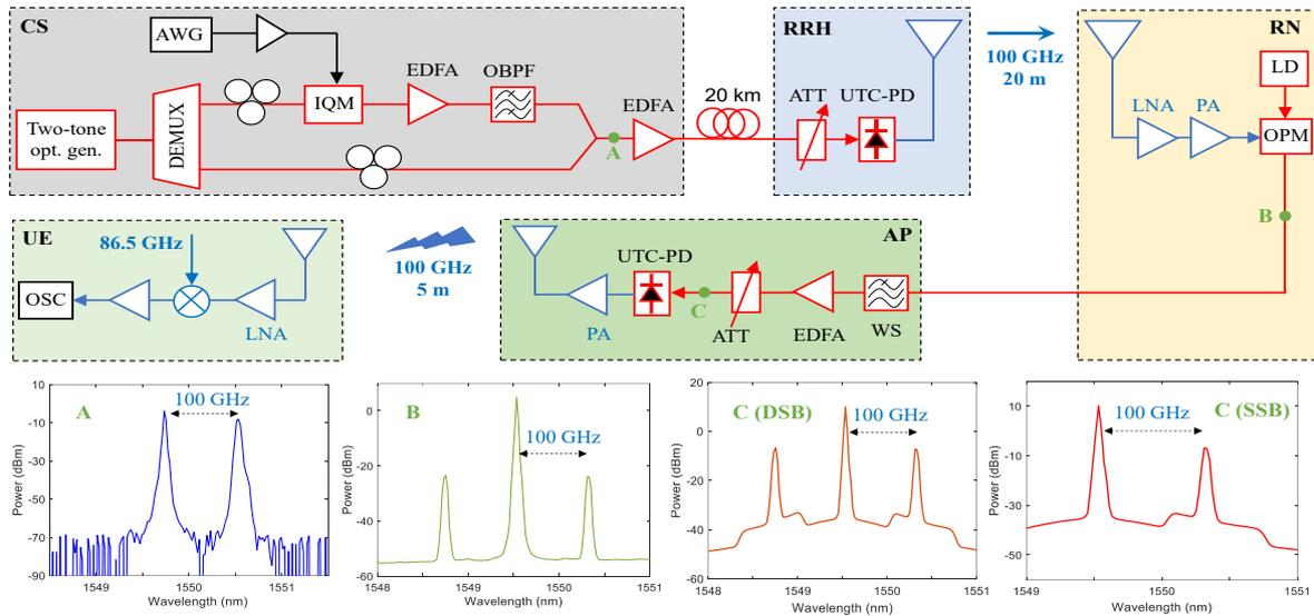
**Fig. 2:** Experimental setup for transparently relaying 100-GHz radio signal to indoor using phase-modulated RoF system.
