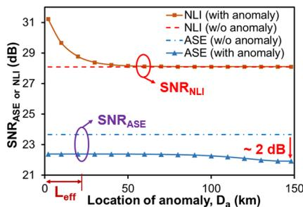
Fig. 3:  $\text{SNR}_{\text{ASE}}$  and  $\text{SNR}_{\text{NLI}}$  depending on anomaly location.
