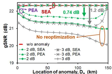
Fig. 4: gSNR depending on location of anomaly loss and mitigation algorithm.
