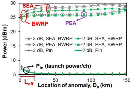
**Fig. 5:** Fiber launch power and BWRP power depending on reoptimization algorithm and location of anomaly loss.
