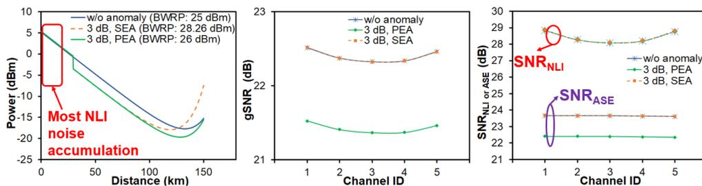
**Fig. 6:** (a) Power profile in fiber, (b) gSNR, (c)  $SNR_{NLI}$  and  $SNR_{ASE}$ .
