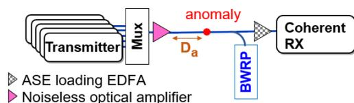
Fig. 1: Transmission system with hybrid Raman amplifier.
