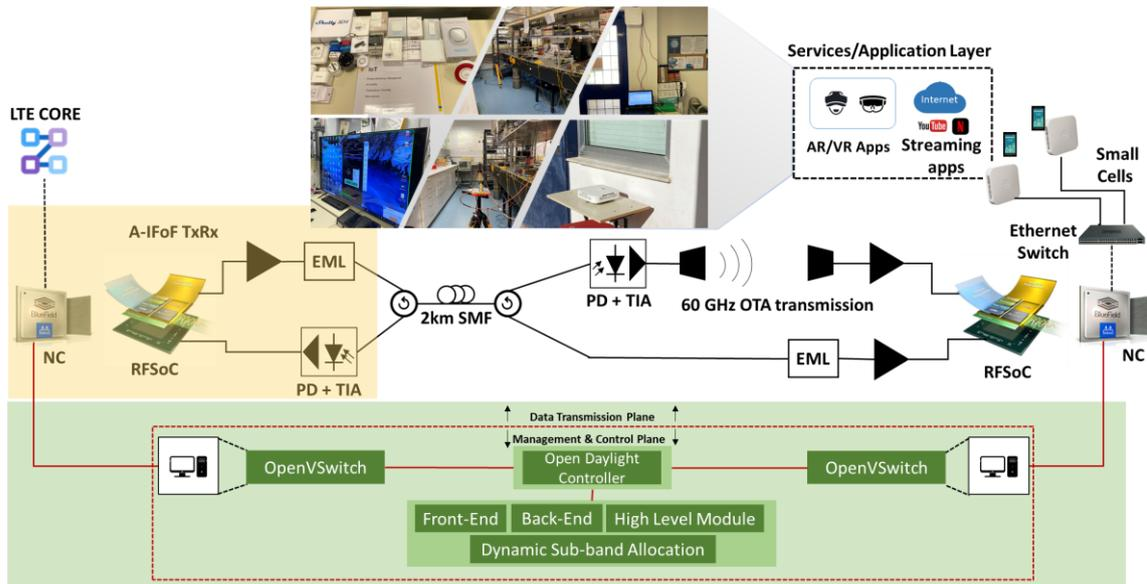
Fig. 1: Experimental Demonstrator layout, involving the Data, Control and Services layers.
