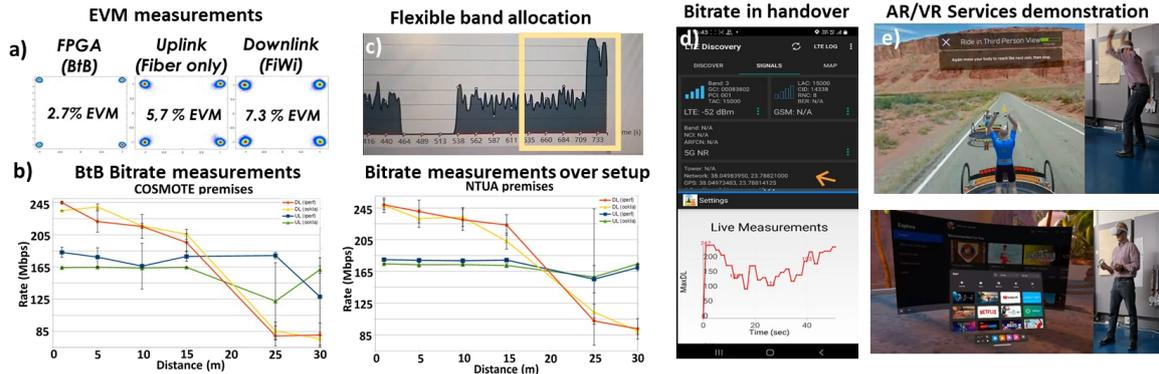
**Fig. 2** a) Constellation diagrams and EVM measurements in Back-to-back (BtB), Uplink (Fiber), Downlink (Fi Wi), b) Bit rate measurements of the transmitted data in both COSMOTE premises (back-to-back) and NTUA (over the deployed infrastructure), c) Demonstration of the dynamic activation of second channel, d) Bitrate measurements captured in the process of handover, e) Demonstrations of AR/VR and streaming services.
