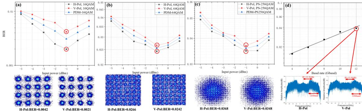
**Fig. 2:** (a) BER of PDM-16QAM signal vs. the input optical power of PD; (b) BER of PDM-64QAM signal vs. the input optical power of PD; (c) BER of PDM-PS-256QAM signal vs. the input optical power of PD; (d) BER of PDM-PS-256QAM signal vs. the baud rate
