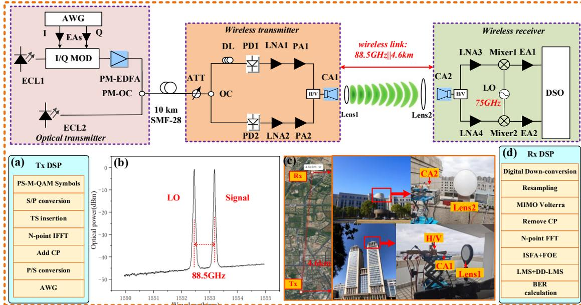
**Fig. 1:** The experimental setup of the photonics-aided W-band polarization multiplexing communication system; (a) block diagram of Tx DSP; (b) optical spectrums of the optical signal after PM-OC; (c) the experimental photos of 4.6km wireless transmission system (Tx and Rx are located between the two campuses of Fudan University); (d) block diagram of Rx DSP
