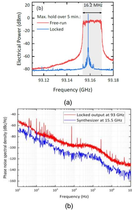
**Fig. 2:** (a) Electrical spectrum of the hybrid laser obtained. (b) Phase noise spectral density of the 93-GHz locked signal and that from the 15.5-synthesizer signal used to drive the Optical Frequency Comb Generator (OFCG)
