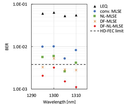
Fig. 6: 224-Gbps/λ 4-ch LAN-WDM PAM-4 performance in 2-km transmission.
