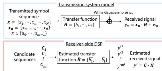
Fig. 1: Concept of transmission system and MLSE.
