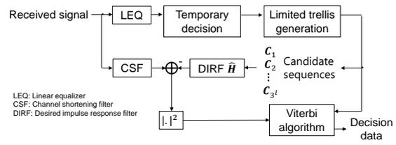
**Fig. 2:** Block diagram of TL-MLSE. (LEQ: Linear equalizer, CSF: Channel shortening filter, DIRF: Desired impulse response filter)
