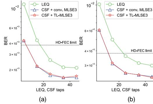
**Fig. 3:** Transmission performance for (a) 225-Gbps 10-km transmission and (b) 255-Gbps 10-km transmission for LEQ (circles), conventional MLSE (triangles) and TL-MLSE (stars).
