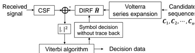
Fig. 5: Block diagram of DF-MLSE with Volterra series expansion.
