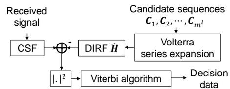
**Fig. 4:** Block diagram of NL-MLSE.
