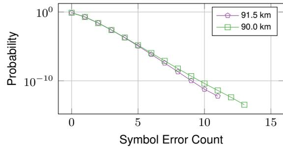
Fig. 6: Probability of corrected codewords for FEC symbol error count
