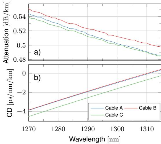
**Fig. 2:** Cable characterisation; a) fibre attenuation and b) chromatic dispersion for cables
