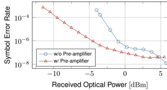
**Fig. 3:** Symbol error rate vs received optical power in back-to-back configuration
