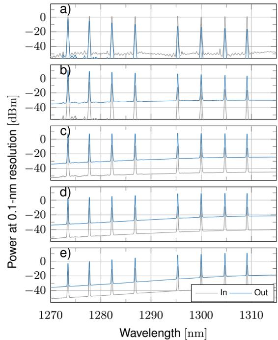
**Fig. 4:** Input/output spectra of a) pre-emphasis filter, b) first BDFAs, c) second BDFAs, d) third BDFAs and e) fourth BDFAs
