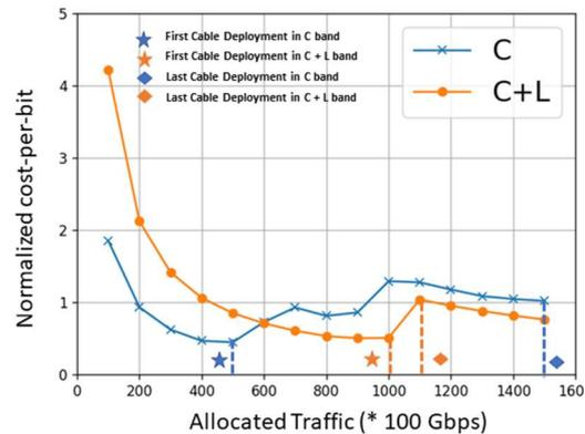
**Fig. 4:** Cost-per-bit variation with traffic loading.
