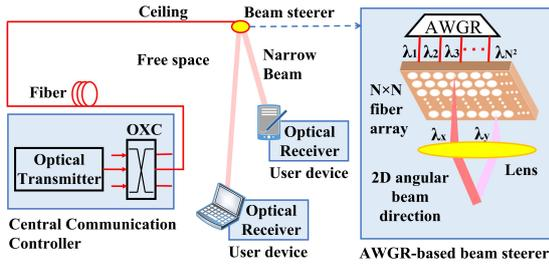
**Fig. 1:** Regular system architecture of the indoor AWGR-based 2D IR beam steering down-link.
