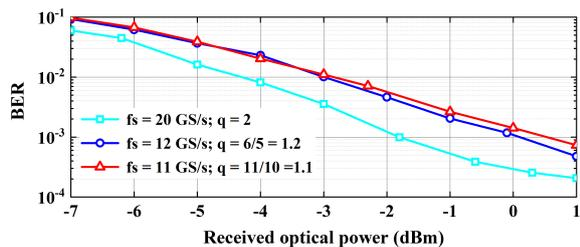
Fig. 4: Measured BER versus received optical power curves with different DAC sampling rates ( $f_s$ ) for a transmission symbol rate of 10 GBaud.
