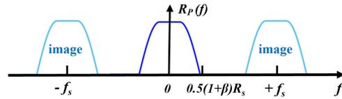
**Fig. 2:** Electrical spectra of the transmitted RRC pulse-shaped signal with oversampling/interpolation.
