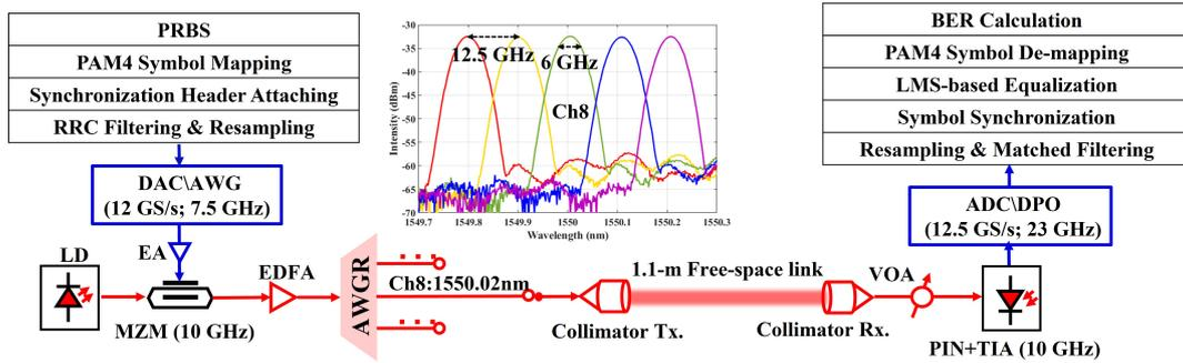
Fig. 3: Experimental setup.
