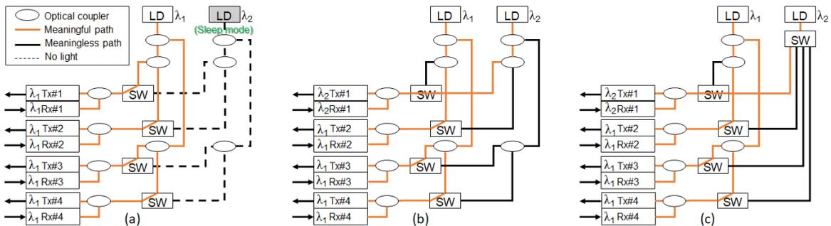
**Fig. 2:** OLT-side LD comunization setup: (a) no failure and secondary link failure cases, (b) primary link failure case with sub-LD light broadening, (c) primary link failure case with sub-LD light switching.
