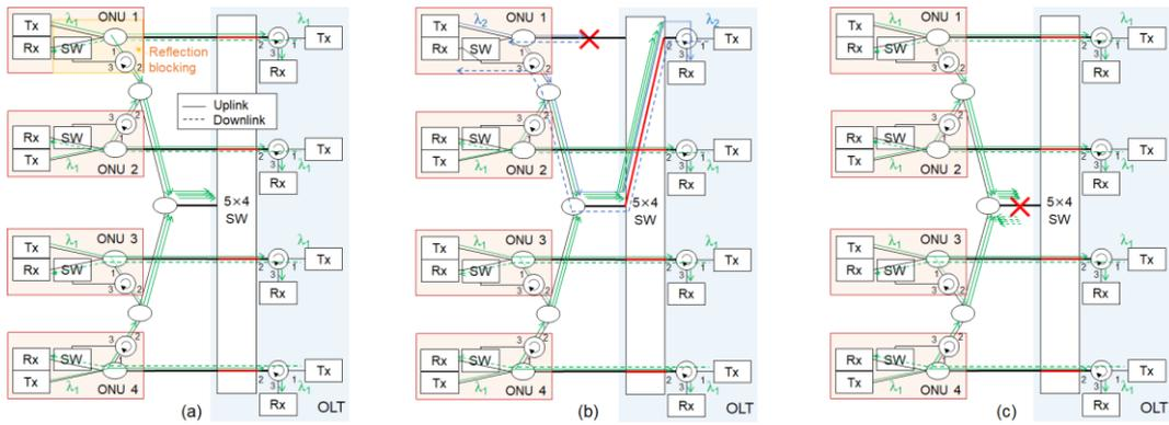
**Fig. 1:** SS/PDS link switchable P-to-MP architecture with edge-side single LD protection: (a) no failure case, (b) primary failure case, (c) secondary failure case.
