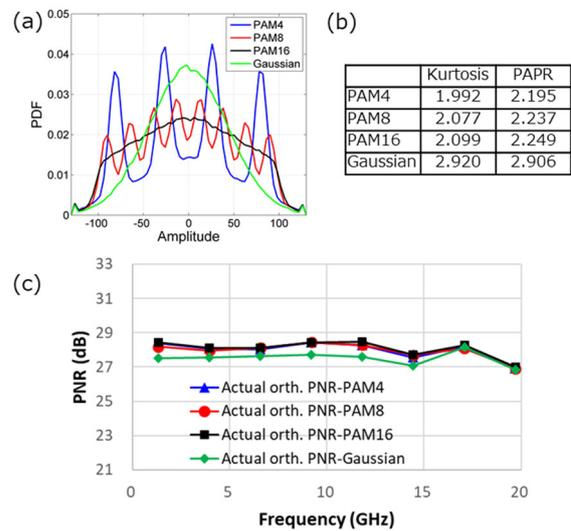
Fig. 5: (a) PDF, (b) kurtosis, and PAPR of four signals with different modulation formats. (c) PNRs of orthogonal noise show that the noise spectrum of DAC and ADC has low correlation with signal PAPR and kurtosis.
