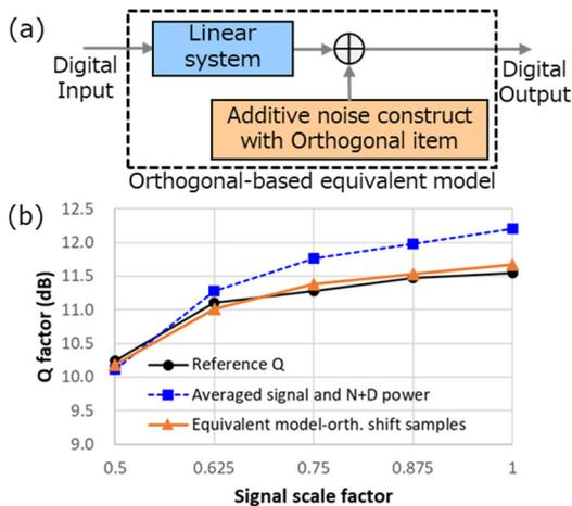
Fig. 4: (a) Equivalent model with additive noise constructed with actual orthogonal term. (b) The estimation results of orthogonal-based equivalent model have similar Q values with actual results.
