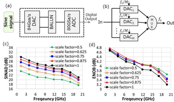
**Fig. 1:** (a) Experimental setup for measuring ENOB and SINAD (b) Schematic picture of time interleaved DAC. (c) and (d) are measured SINADs and ENOBs with different input signal amplitudes.
