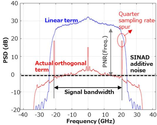
Fig. 3: Power spectrum density (PSD) of linear part, actual orthogonal term, and SINAD constructed AWGN.
