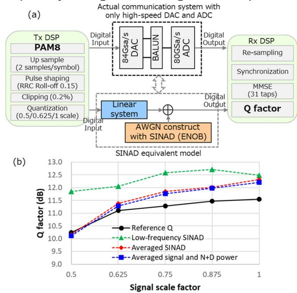
**Fig. 2:** (a) Experimental setup and DSP flow of actual communication system, and the equivalent model based on common understanding of SINAD. (b) Comparison between actual Q factors and SINAD estimated Q factors.
