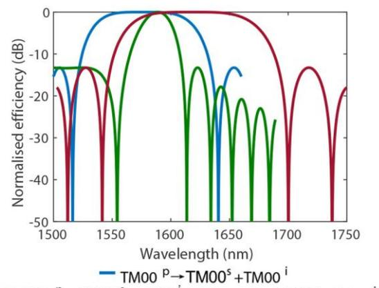
**Fig. 1:** Calculated normalised efficiency of three parametric processes as a function of wavelength in a multimode PPLN waveguide (blue: intramodal TM00-mode DFG; green: intermodal DFG; red: intramodal TM10-mode DFG).
