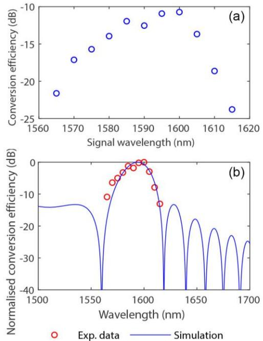
**Fig. 4:** (a) Conversion efficiency measured at different input signal wavelength; (b) measured and calculated normalised conversion efficiency.
