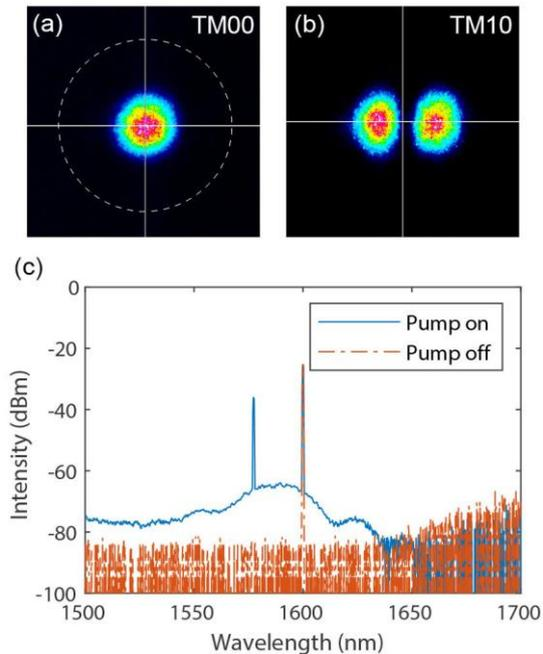
**Fig. 3:** Images of (a) the throughput signal beam and (b) the idler generated from the intermodal DFG process; (c) output spectrum measured from the multimode fibre.
