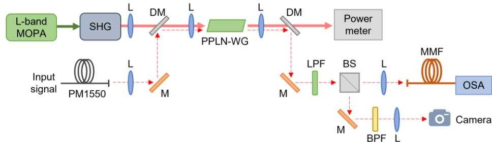
**Fig. 2:** Schematic of the intermodal DFG experiment. BPF: band pass filter; BS: 50:50 beam splitter; DM: dichroic mirror; L: lens; LPF: long pass filter; M: mirror; MMF: multimode fibre; MOPA: master oscillator power amplifier; OSA: optical spectrum analyser; PPLN-WG: periodically poled lithium niobate waveguide; SHG: second harmonic generation.
