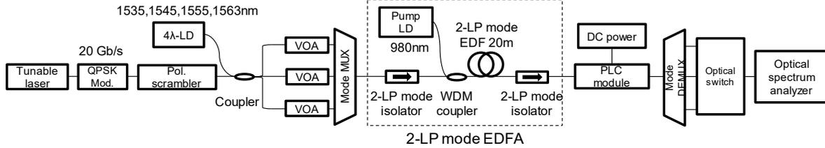
Fig. 4: Experimental setup for variable DMG equalization of two-LP mode EDFA.
