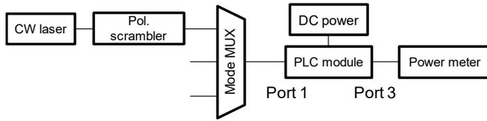
Fig. 2: Experimental setup for measuring modal loss property of fabricated PLC module shown in inset photo.
