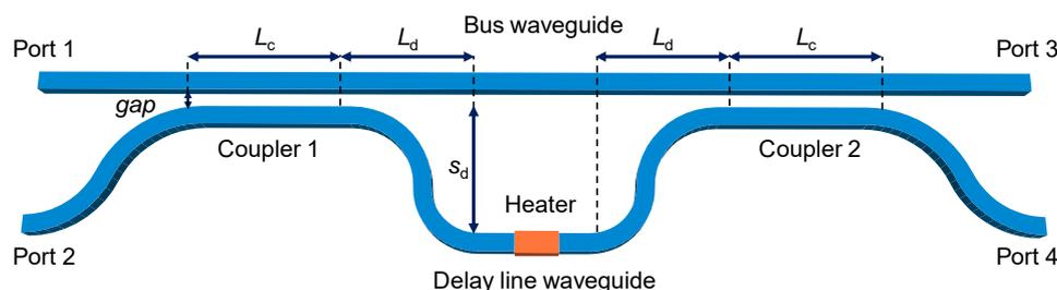
Fig. 1: Schematic of proposed two-LP-mode variable MDL equalizer.
