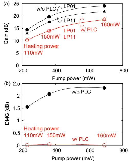
Fig. 5: Pump-power dependence of (a) gain and (b) DMG measured at 1550 nm.
