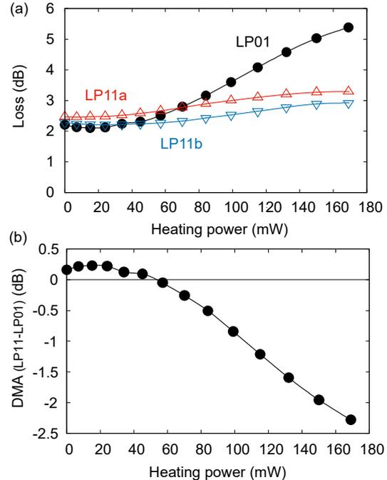
Fig. 3: Measured (a) loss and (b) DMA at 1550nm as function of applied power to heater.
