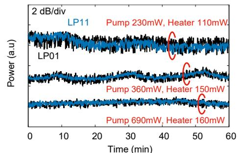
Fig. 7: Time variation of output power of PLC module measured at 1550 nm.
