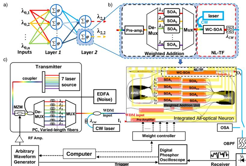
Fig. 1: (a) All-optical neural network. (b) SOA-based all-optical neuron. (c) Experimental setup.
