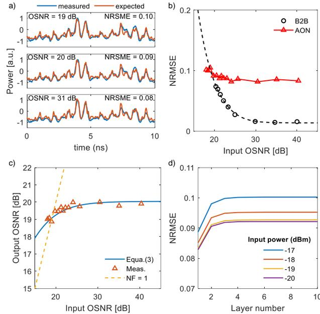
**Fig. 1:** 7-channel input to 1 output AON: (a) Measured (blue) and expected (red) time traces at the output (b) Error vs. the input OSNR for back-to-back (circles) and AON testing (triangles). (c) Output OSNR vs. input OSNR from equation (3) (blue line), measurement (triangles) in (b), and  $NF = 1$  (dashed line). (d) Optimization with tuning the input power per channel.
