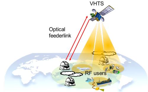
**Fig. 3:** High-throughput satellite concept with optical feederlink.
