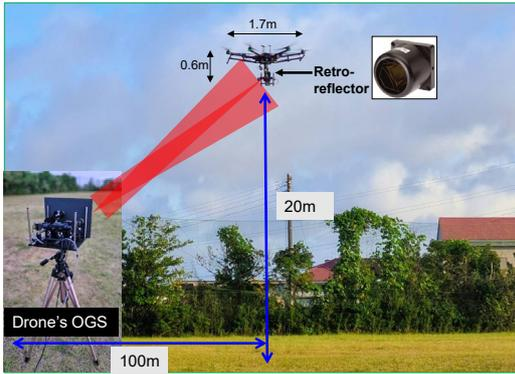
**Fig. 2:** Free-space optical link between a hovering drone and a simple optical ground station
