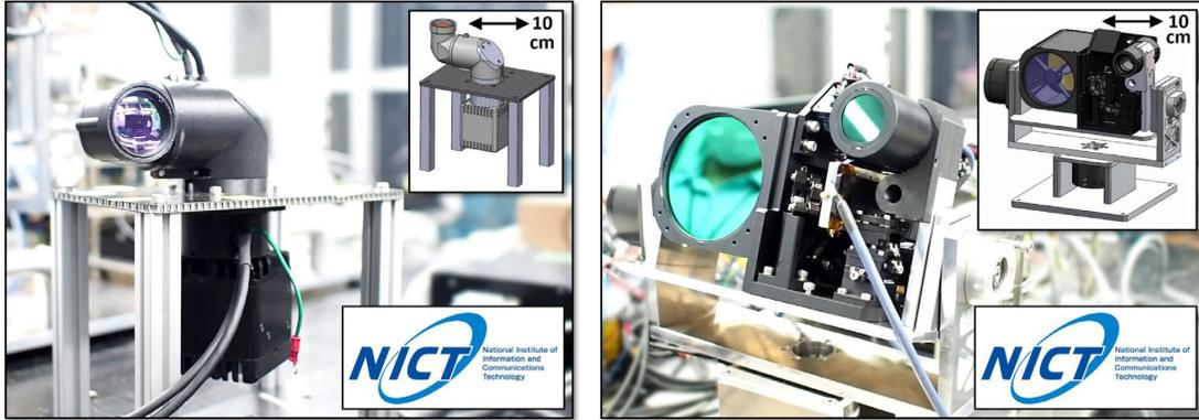
Fig. 1: Early prototypes of ST terminal (left) and FX terminal (right) for preliminary validation.
