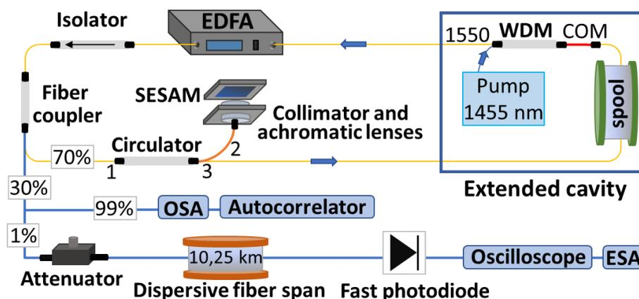
**Fig. 1:** Schematic of the setup for the characterization of ultralong pulsed fiber lasers, where the extended cavity can take different lengths.
