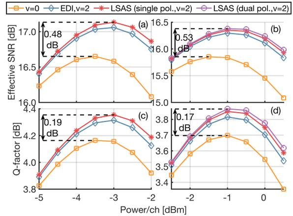
Fig. 2: Effective SNR (a,b) and Q-factor (c,d) vs. launch power. (a,c): Single pol. (b,d) dual pol. CCDM with  $L = 180$ .
