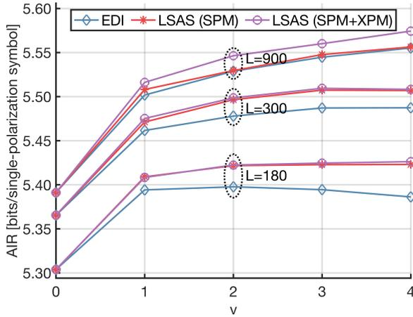
Fig. 1: AIR vs.  $v$  for different CCDM blocklengths  $L$ .
