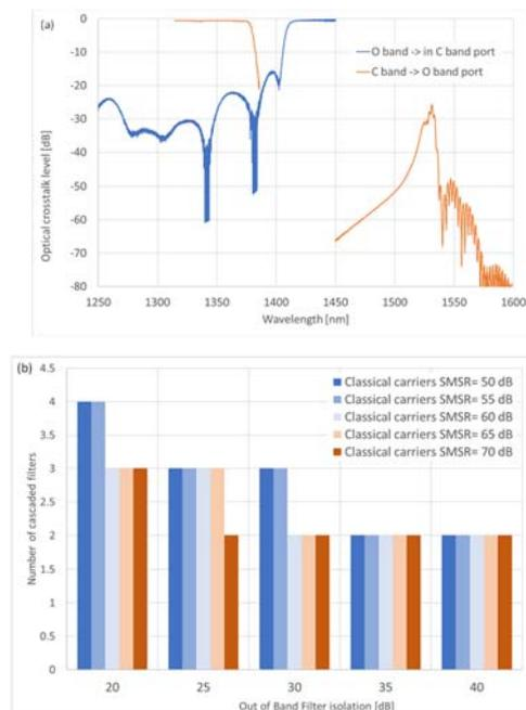
**Fig.2:** (a) Optical Out of Band extinction for O/C band splitters/combiners, (b) Estimation of the number of filters to be cascaded to guarantee spectral extinction.
