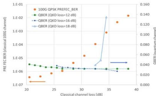
**Fig. 4:** BER against loss for classical and quantum carriers over 20 km of G.652 fiber (blue and green curve for QKD carrier, orange for classical one).
