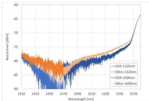
**Fig. 3:** Raman noise after 50 km of fiber (orange trace) compared to no fiber transmission (blue curve).
