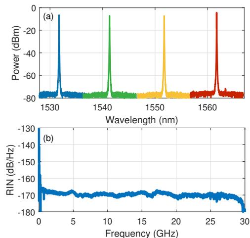
**Fig. 1:** (a) Superimposed spectra of the optical carrier used in this demonstration using the DLM and (b) the typical RIN of the DLM optical carrier at 1551.12 nm.
