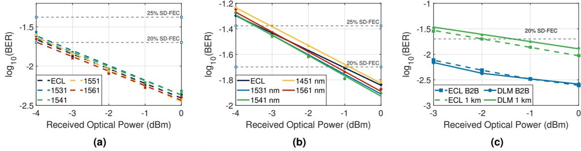
**Fig. 4:** BER performance of 32 GHz 32QAM-OFDM signal in (a) B2B and (b) after 1 km SMF transmission, evaluated at various wavelength across C-band, and (c) BER performance of 40 GHz 16 QAM-OFDM signal.
