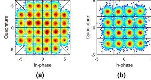
**Fig. 6:** Scatterplot of (a) 32 GHz 32QAM-OFDM and (b) 40 GHz 16 QAM-OFDM signals after 1 km SMF transmission.
