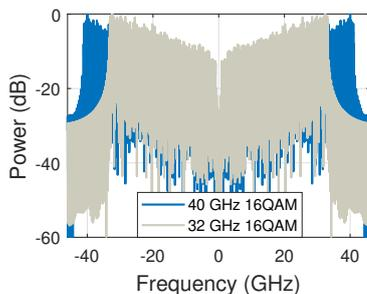
**Fig. 3:** Spectrum of the 32 GHz and 40 GHz signal at the transmitter with digital pre-distortion.
