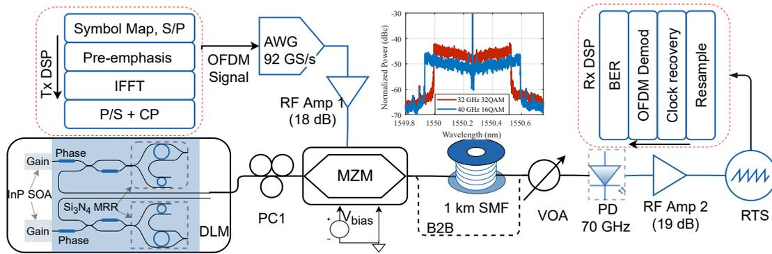
**Fig. 2:** Schematic of the experimental setup for the demonstration of wideband OFDM transmission using InP-Si<sub>3</sub>N<sub>4</sub> laser.
