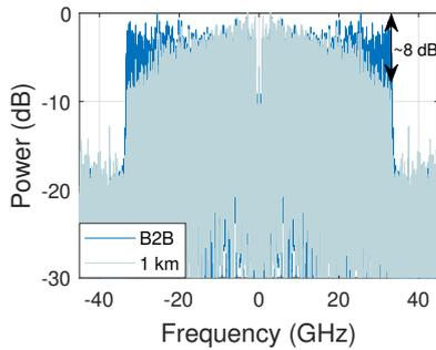
**Fig. 5:** Effect of dispersive fading on the spectrum of the received 32 GHz signal after 1 km SMF transmission.
