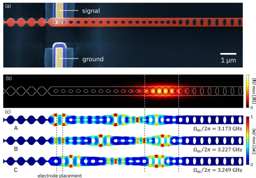
**Fig. 1:** (a) False-color scanning electron microscope image of a GaP photonic crystal cavity suspended above integrated niobium electrodes. (b) Finite-element-method (FEM) simulation of the localized optical mode. The color scale indicates the magnitude of the electric field  $|E|$ . (c) FEM simulation of three extended mechanical breathing modes. The color scale indicates the magnitude of the mechanical displacement  $|u|$ .
