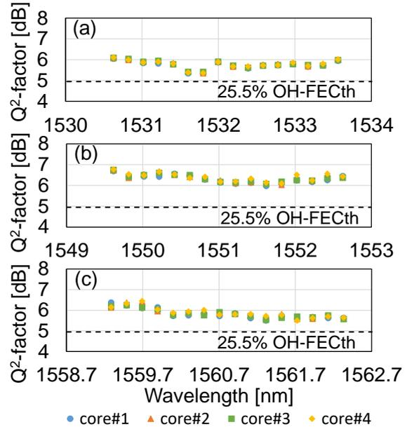
Fig. 4: Q<sup>2</sup>-factors for all 4-SDM/16-WDM channels after 7,000-km transmission at approximately (a) 1532 nm, (b) 1551 nm and (c) 1560 nm in the bidirectional case.
