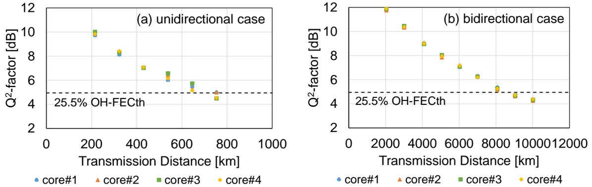
Fig. 3: Q<sup>2</sup>-factors as a function of the transmission distance in the (a) unidirectional case and (b) bidirectional case.
