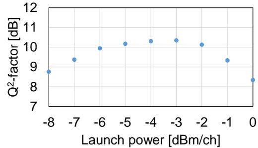
Fig. 2: Q<sup>2</sup>-factors as a function of the fibre launch power after 3,015-km transmission.
