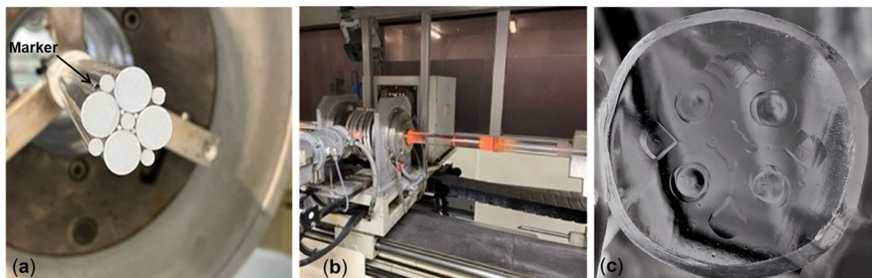
Fig. 1: Assembly of core-rods, adjusting rods and marker to make the stacked primary preform (a); bench on which the stacked primary preform is collapsed (b); cross-section of the collapsed primary preform (c).
